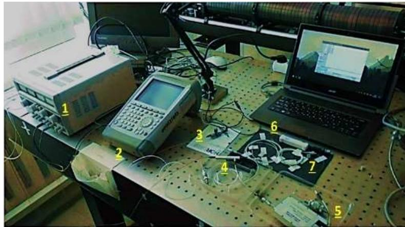
Fig. 4. Universal setup for microwave photonics experiment: 1 – DC power supply, 2 – spectrum analyzer, 3 – narrow-band laser, 4 – PM, 5 – microwave signal generator, 6 – MZM modulator, 7 – photodetector [15]
